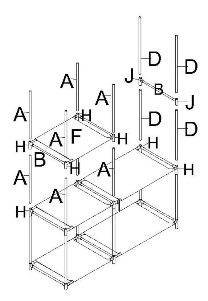
Repeat step 2 for the left shelf one time, and insert tube (D) into part (H), assemble tube (B&D) through part (J) on right shelf.
