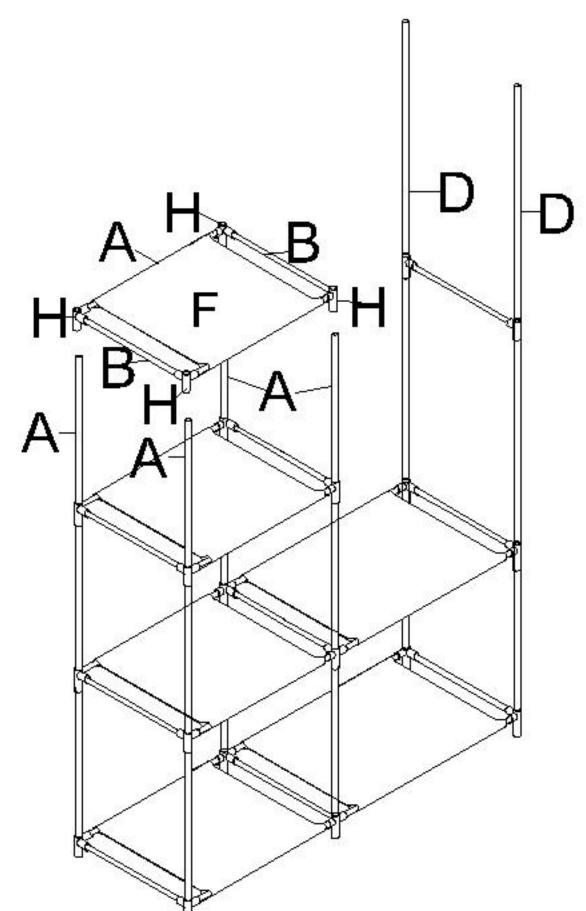
Attach fabric(F) into tube(A), assemble tube (A&B) with part (H). then assemble this assembled frame to tube (A).
