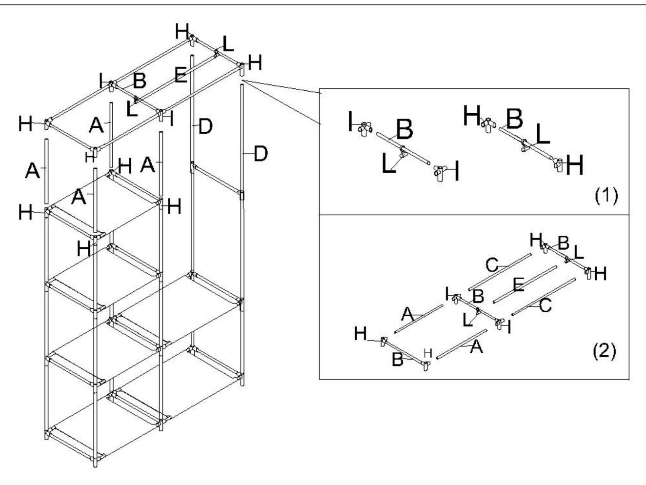
First, insert hook (L) to tube (B), assemble part (H&I) to part(B), then insert tube (E) into hook (L). Repeat step 1 without the layer fabric, then insert fixed frame on tube (A&D).
