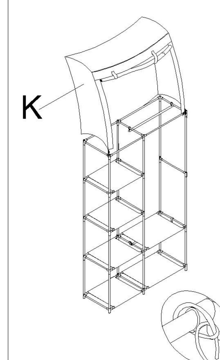
Put cover fabric (K) to the whole finished construction, then fasten with ropes
