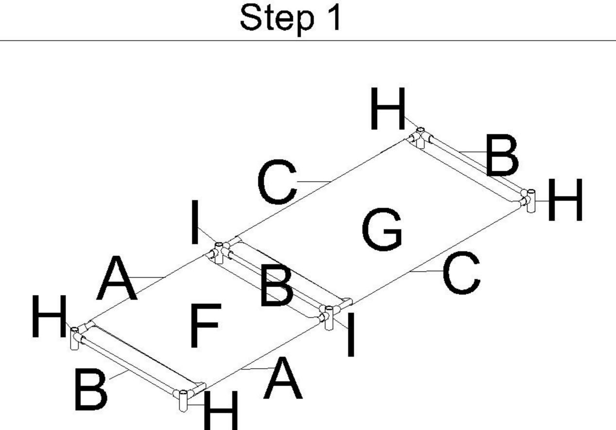
Attach fabric (F) into tube (A), attach fabric (G) into tube (C), assemble tube (A&B&C) with part (H&I). Repeat one time.
