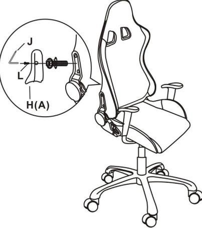
Install back, first screw the upper screws of two sides to fix the back, then screw the rest two.
